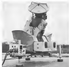
TARGET TRACKING RADAR (left) is a three-axis unit developed by Erlangen firm MELLE. Aperture at right of dish is for conventional reference sensors used to check automatic tracking, or for manual tracking. Beam-riding tube (right) in the foreground can, with both coarse and fine focus beam control systems. Coarse focused sections rotate coarse focus, dish and beam tube transmit the fine focus. Aperture is shown for the data collection in mobile flight path.
